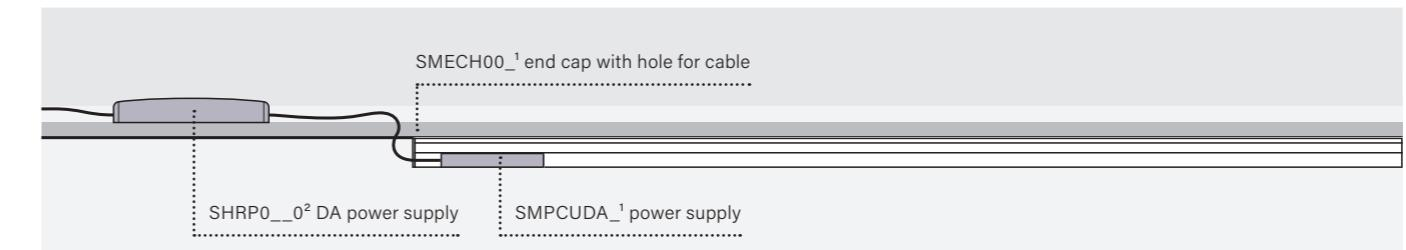
suspended multitrack + recessed power supply
