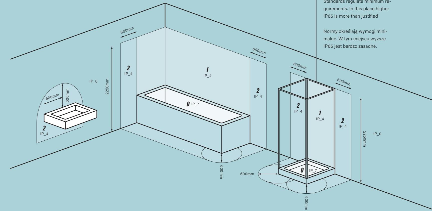
Standards regulate minimum requirements. In this place higher IP65 is more than justified
