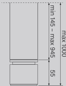
In the PET next rift system, you select a lighting module that has fixed dimensions (visible height: 55mm) and you configure the rest of the luminaire separately: the housing module.
