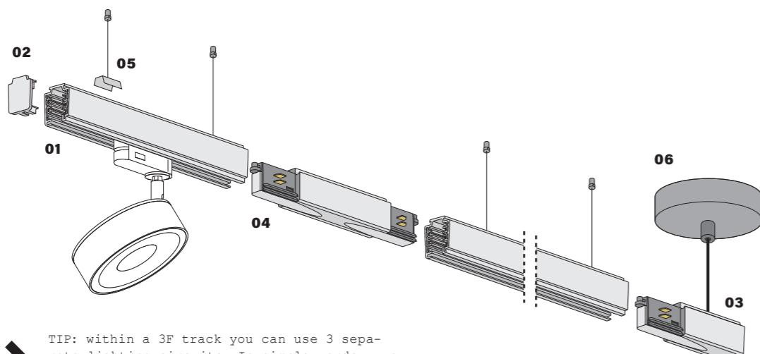
**TIP:** within a 3F track you can use 3 separate lighting circuits. In simple words - you can create 3 separate lighting scenes easily!
