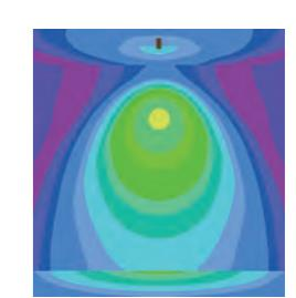
**50°** – is the angle for general purpose lighting or when a luminaire is mounted in the proximity of the illuminated object.
