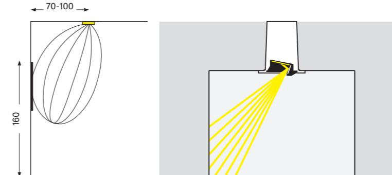
Light emitted by RAFTER wall washer is reflected by tiny mirror which is integrated with luminaire optics. As a result, the light is directed to wall instead of the floor even though luminaire is almost flushed with the ceiling surface.
