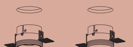
PUTT trimless version allows to pull out the inner ring by 10mm. It is possible before and after assembly.
