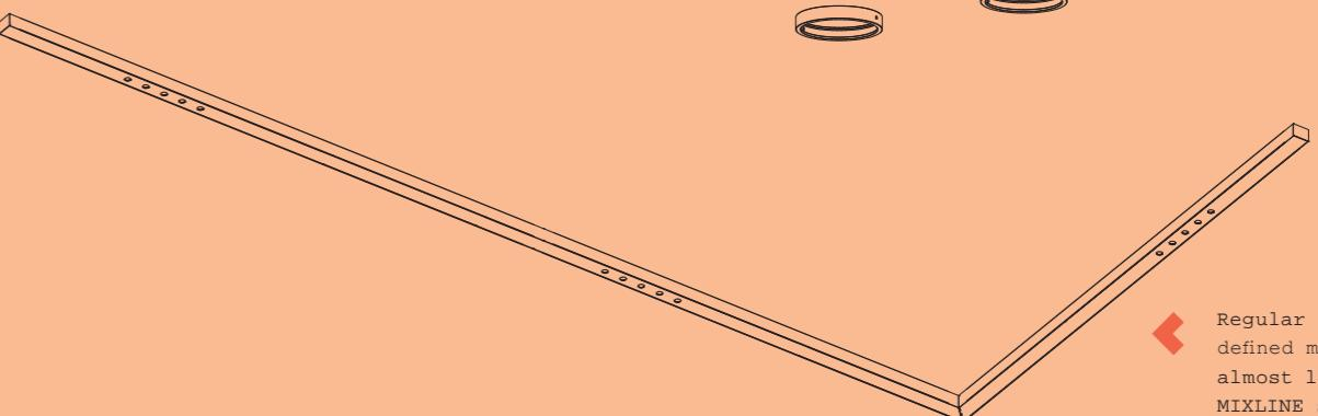
Regular systems have previously defined modules which you can arrange almost like a puzzle! Like in shown MIXLINE system where several modules with points were joined with an angular connector to get a long profile for reception desk which has its working spaced angled.
