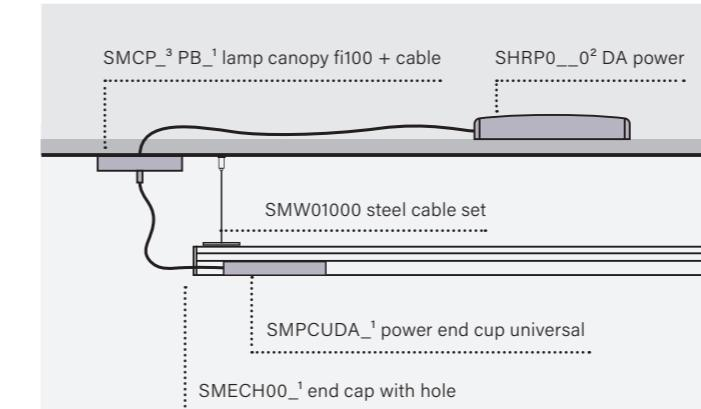
suspended multitrack + surface power supply
