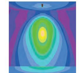
**18°** – the appropriate angle when the luminaire is mounted at a longer distance from the illuminated surface or if we would like to obtain a strong chiaroscuro effect. A narrow angle will prevent light from "reaching the target". It can be used only as task or accent lighting.
