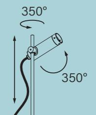
You can easily adjust the height and the angle of the DART head.
